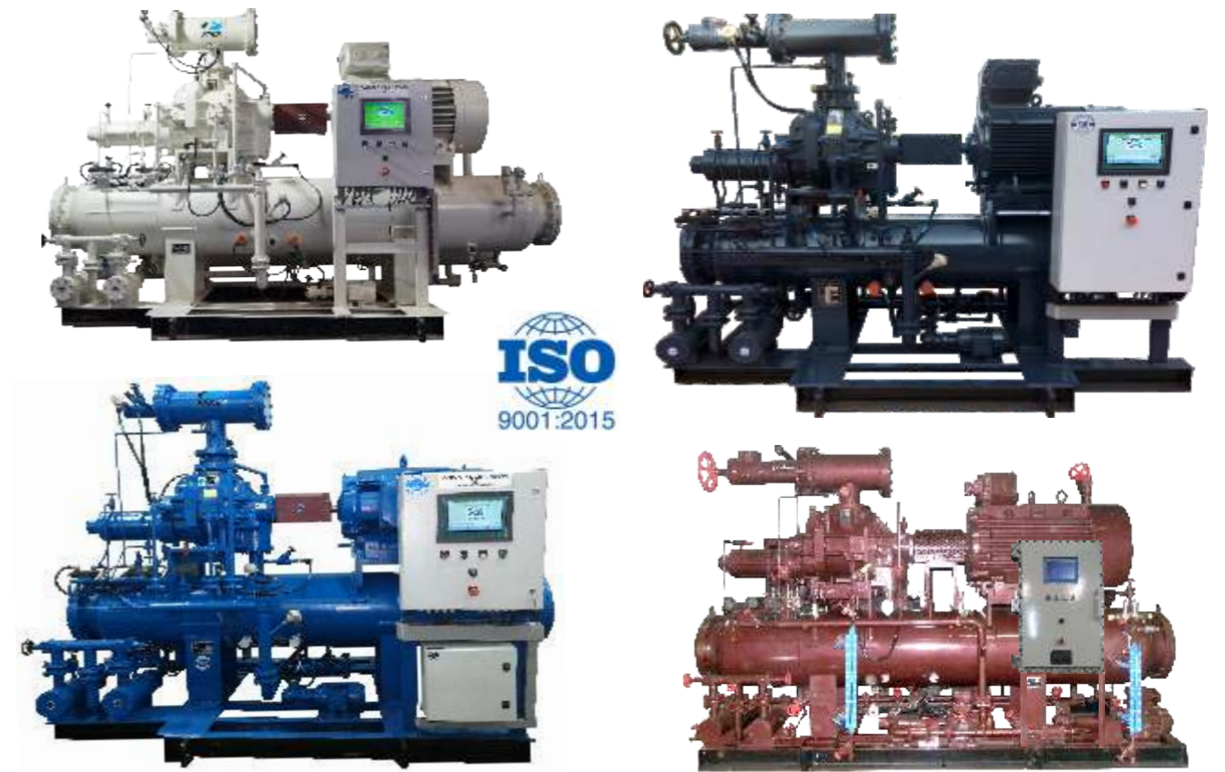
Frick India Rotary Twin Screw Compressor Package with Horizontal oil Separator using MBM Series Screw Blocks Capacity Range : 404 Kw to 3300 Kw (521m3/hr to 4089m3/hr.) @23 Deg F SST & 104 Deg F CST
